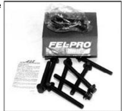
Fig. 4. A new set of cylinder head bolts is cheap insurance against a comeback. The set above is for a Quad 4 and was obtained at a local jobber for under 20 bucks.
