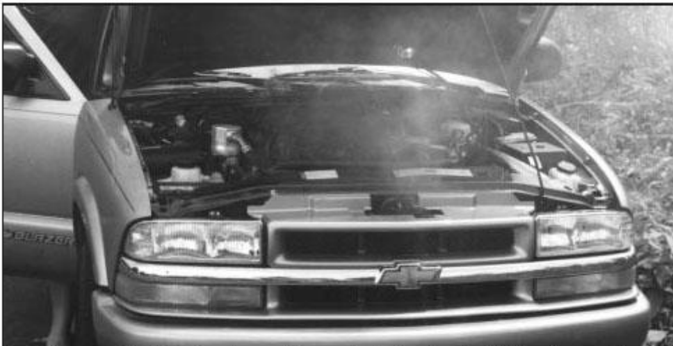
Even the newest vehicle is not exempt from cylinder head gasket failure. Incorrect installation from the factory or disregard for manufacturers guidelines on operation and maintenance can produce the pictured result.
